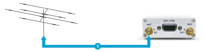
1. Connect antenna to the receiver's antenna input.
