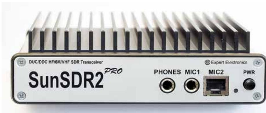
PHOTO 1: SunSDR2 PRO – front panel connections.
