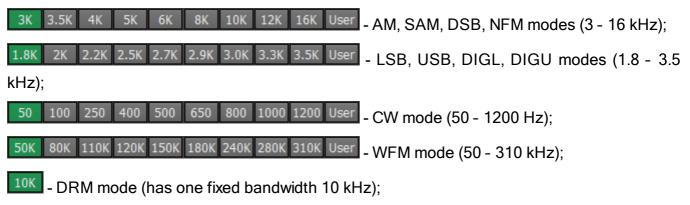
user can adjust the RX filter bandwidth by himself (available at any modulation type except DRM).
