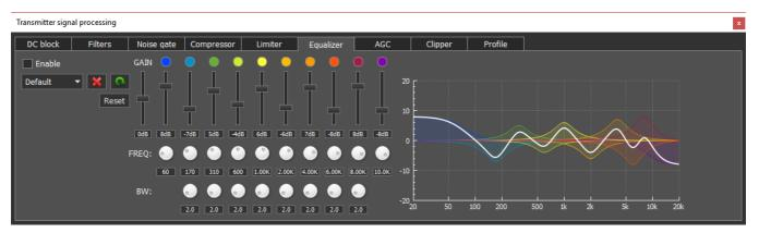
Parametric equalizer module with graphic display of the summed AFC (white line) and AFC of each equalizer. Each equalizer has independent set of controls: the center or primary frequency (**FREQ**), bandwidth (**BW**) and AFC level (boost or cut) - vertical slider. Press right mouse button on any control element to set it to the default value. Thus, using the parametric equalizer you can perform the finest tuning on any required frequency.
