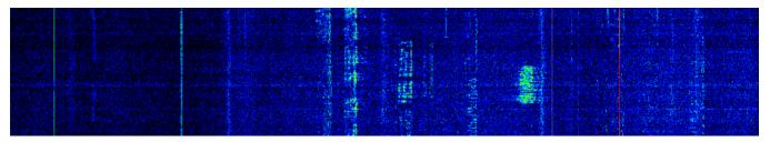
Waterfall graphic - timed spectrum scope in the format: amplitude - brightness, frequency - horizontal, time - vertical. The comfortable settings are set by default, but you can change them if necessary (more details in <u>Waterfall tab</u><sup>D75</sup>).
