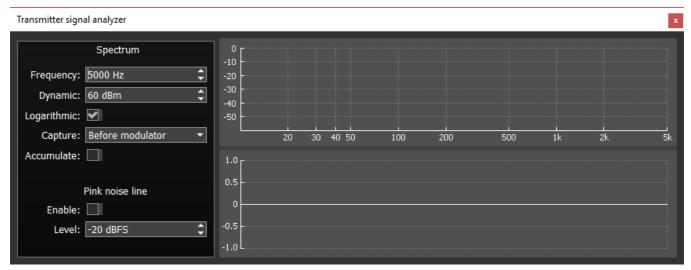
Frequency - top limit of the horizontal (frequency) scale of the transmitter.
