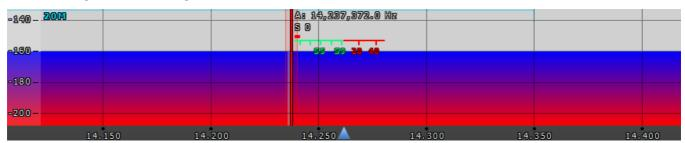
In this window, you can see the spectrum, with the sample rate from 39 up to 312 kHz (adjustable by User) and the RX filter to tune and listen to the stations.
