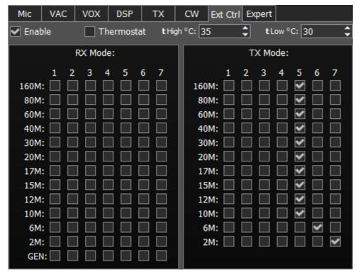
Enable - checkbox to enable control of the electronic keys.
