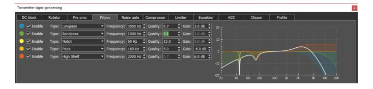
**Parametric filter module** with graphic display of the summed AFC (amplitude-frequency characteristic - white line) and AFC of each filter. Simultaneously you can use up to 5 filters. Available filter types:
