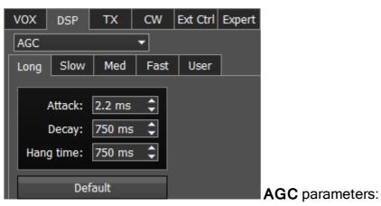
**Attack** - when a signal gets stronger, this value determines how quickly the AGC will decrease gain.
