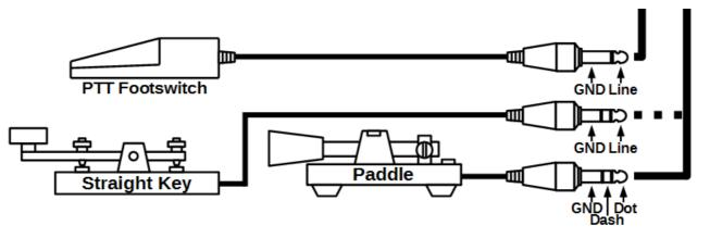
You can connect several accessories to the transceiver's rear panel, as shown on the picture above.
