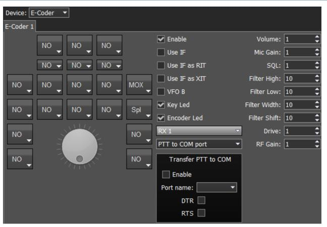
In the left part of the menu you can see the schematic picture of the E-Coder panel with buttons and knobs. Press any button, you'll see the list of the available functions.
