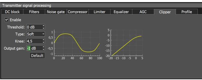
**Clipping** is a form of waveform distortion that occurs when the output Voltage exceeds **Threshold**. Visually (on oscilloscope) it looks like altered signal peaks, you can hear it as splutters and cracks. **Clipper** reduces signals peak-factor and increases overall power, but distorts the signal.
