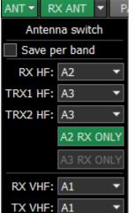
**TXVHE:** A1 - Antenna switch menu. This menu allows you to lock the required HF/VHF antenna input only for RX. When the certain HF/VHF antenna input is locked for RX you cannot select it for TX.
