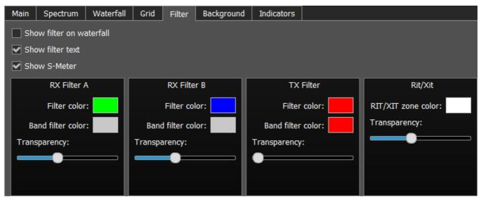
• Show filter on waterfall - Show receiver(s) filter on the waterfall. Set the Show filter on waterfall checkbox to show receiver(s) filter on the waterfall.
