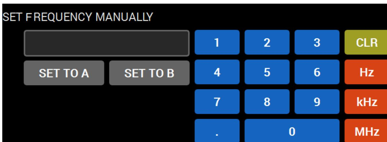
Enter the required frequency either with touchscreen or with physical buttons on the front panel, then apply the entered frequency either to VFO A (SET TO A) or to VFO B (SET TO B).
