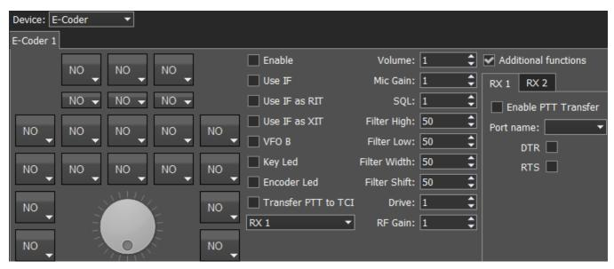
In the left part of the menu you can see the schematic picture of the E-Coder panel with buttons and knobs. Press any button, you'll see the list of the available functions.
