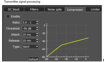
Compressor - is used to reduce
