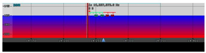
The panorama consists of two parts separated by the horizontal scale: 1) Spectrum Scope and 2) Waterfall.
