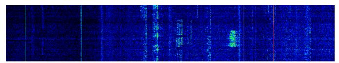
Waterfall graphic - timed spectrum scope in the format: amplitude - brightness, frequency - horizontal, time - vertical. The comfortable settings are set by default, but you can change them if necessary (more details in Waterfall tab<sup>\(D\)62</sup>).
