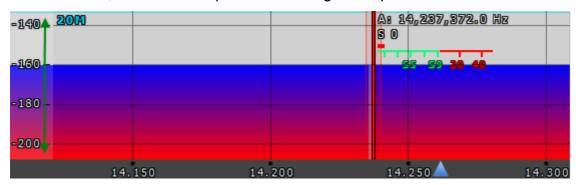
The horizontal scale between the spectrum scope and waterfall shows the frequency of the certain point on the spectrum. If you move the mouse cursor over the horizontal scale a hand will appear. Press and hold the right mouse button, then move it left/right to zoom in/out the panorama or press and hold the left mouse button, then move it up/down to change the ratio of the spectrum to waterfall.
