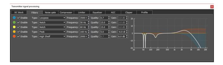
Parametric filter module with graphic display of the summed AFC (amplitude-frequency characteristic - white line) and AFC of each filter. Simultaneously you can use up to 5 filters. Available filter types:
