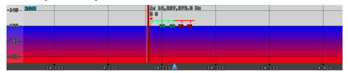
In this window, you can see the spectrum, with the sample rate from 48 up to 960 kHz (adjustable by User) and the RX filter to tune and listen to the stations.
