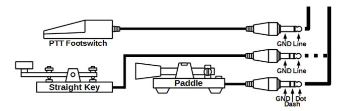
You can connect several accessories to the transceiver's rear panel, as shown on the picture above.
