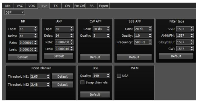
**NR** - Noise Reduction, removes the white noise. This is a special adaptive filter, which removes any abnormal noises from the air in the RX filter band.
