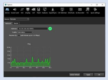
After starting the program, the radio can be found on the internet and can then be remotely controlled as a receiver and transmitter. Access works under LAN, WLAN, LTE and 3G/4G/5G.
