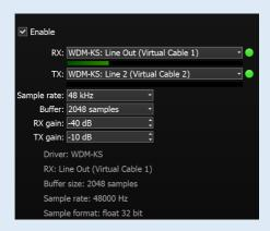
In Options>Device>VAC set the RX to VC1 and TX to VC2. The sample rate is 48000Hz. Keep the gain settings at the default 0dB for the time being. They may need to be adjusted later if JTDX or WSJTx is used. Buffer here is set at 2048 samples in VAC version 4.64 but some users successfully use 256 samples. The lower size means less latency but can give rise to audio artifacts.
