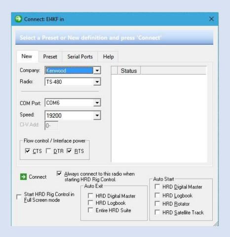
The CAT protocol ECATv1 is equal to Kenwood TS-480. If you find that HRD has difficulty connecting, try increasing the Speed (Baud Rate) to 115200 with only RTS checked. The mismatch in Baud Rate does not matter so long as you set 'emulate baud rate' in VSPE. Later versions of HRD appear to have this bug fixed.
