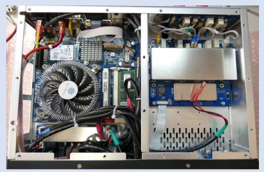
1. HPF should be installed between antenna switch and SDR board. Detach the blue cable (VHF OUT).
