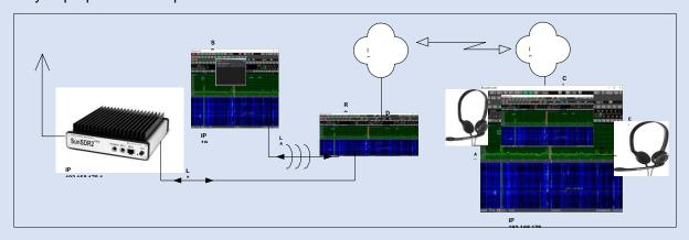
A server / client connection is required for remote control via the internet. Any PC / laptop in the home can act as a server. From <a href="https://eesdr.com/en/software-en/expertremote-en">https://eesdr.com/en/software-en/expertremote-en</a> the remote server and remote client software can be downloaded. Install on the remote and local PCs.
