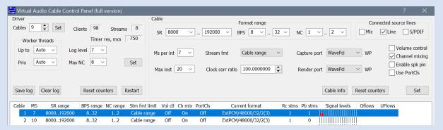
After changing Cable 1, press 'Set' (next to Reset Counters). Do the same with Cable 2. Finally, at the bottom of the VAC Panel (not shown) press Restart Audio Engine. If you get an error here it is because you did not run the Panel 'As Administrator'.
