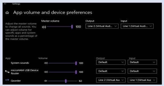
For non-contest recording, at times when you are not using N1MM+ for example, the Hot-Key CTRL+ALT+O will save the current audio buffer to a file in your AUDIO\_YYYY directory. Whatever your radio is hearing, QSOrder will record 45 seconds of audio.
