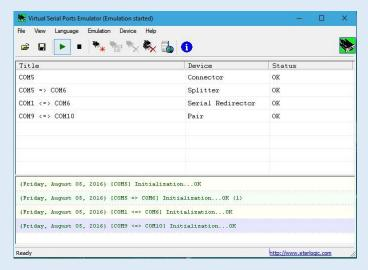
In VSPE redirect COM 6 so that it transfers data from COM 5 to COM 1 (the physical hardware port on the MB1). Go to Device > Create >
