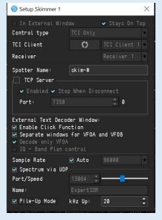
Sample Rate of the Skimmer can be set manually or set to Auto so that it always matches the sample rate of the SDR.
