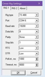
The ESDR\* CAT emulates the Kenwood TS-480 protocol. The application end of our COM port pair for CAT is COM 6. We set the baud rate at 19200 in ESDR\*. Initially set RTS and DTR to Low but, in the event of a connection failure, try with High. Once configured, click OK which will save the configuration.
