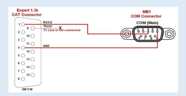
By virtue of having redirected COM 6 to COM 1, the MB1 hardware port now carries CAT data. It can be used for connecting to another computer, via a null modem cable, or to an external device CAT port. For a CAT controlled amplifier, a fully wired null modem cable is
