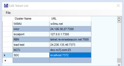
This is then selected in the N1MM Cluster List as the Cluster for N1MM to use. Set 'Automatically Logon' so that a connection is made when N1MM starts. The output from the external Clusters defined in SDC, together with the SDC Skimmer, will be sent to N1MM.
