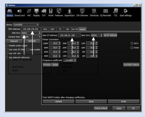
Left, where to set the radio IP address for use on a home network. See text above. Enter the new address and press OK to confirm. After saving the data, switch off the radio, disconnect the Ethernet cable from the PC and reconnect to the
