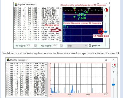
This screen snapshot is when run with WriteLog's unlimited version.
