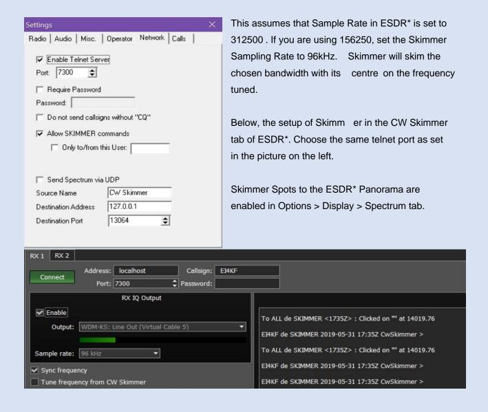
The Features tab in ESDR\* Options can be used to launch CW Skimmer when starting ESDR\*.
