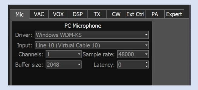
If using ESDR\* version 1.3 there is now no separate PC Microphone setup. The VAC Line 10 input would need to be put in the Soundcard setting. See section 6.19 – Line 10 is set where Line 9 is shown there.
