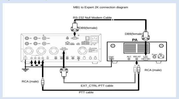
ALC is not connected. As at ESDR2 1.3.1 Update 8, ALC has not yet been implemented. In ESDR\*, for PA control, turn on PA and set up PA PTT in Options. Avoid hot-switching by setting a delay of at least 5ms. The headings X8, 1, 2, 3, 4 refer to the PTT connectors on the MB1 rear panel.
