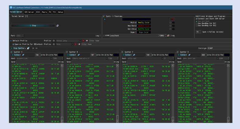
The Telnet Server, as seen above with left half at top, is used to select which local and external Cluster servers are used and how the incoming data is distributed. It also determines globally whether Spots go to the Panorama, whether the SDC Skimmer(s) are active, Spot colours, and if additional windows BandMap(s) and ActiSpot are displayed. Enter your callsign in the Callsign box, seen in right half, lower picture.
