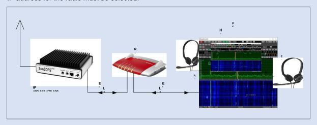
First of all, determine a free IP address on the router. Example, if the router's own address is 192.168.0.1 and it is allocating DHCP (automatic IP assignment) in the range 192.168.100 to 192.168.0.200 then select a free address below .100 as a static address (example 192.168.0.99). Enter this into the ESDR\* software. The SDR port of 50001 is set at the factory and should not be used by any other software on your network. See the Troubleshooting section if this is not the case.
