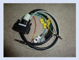
The USB CW Keyer also has a CAT output (and the cable for it is less complex and cheaper to buy). These devices connect to a USB port, either on the MB1 or on an external computer which then gives a CAT feed to that machine. COM port configuration is done by the MicroHam Device Router software.
