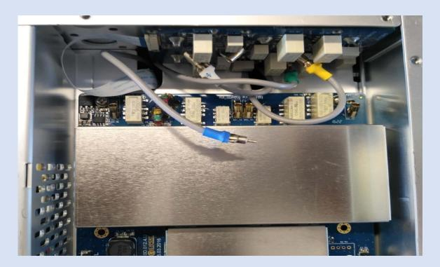
On the back of the HPF board you can see sticky surface, you should attach the HPF to the shield with it, as shown below.
