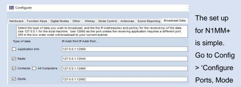
Control, Audio, other' and open the Configurer. In the Broadcast Data tab, enable Spots with an address:port of 127.0.0.1:12062
