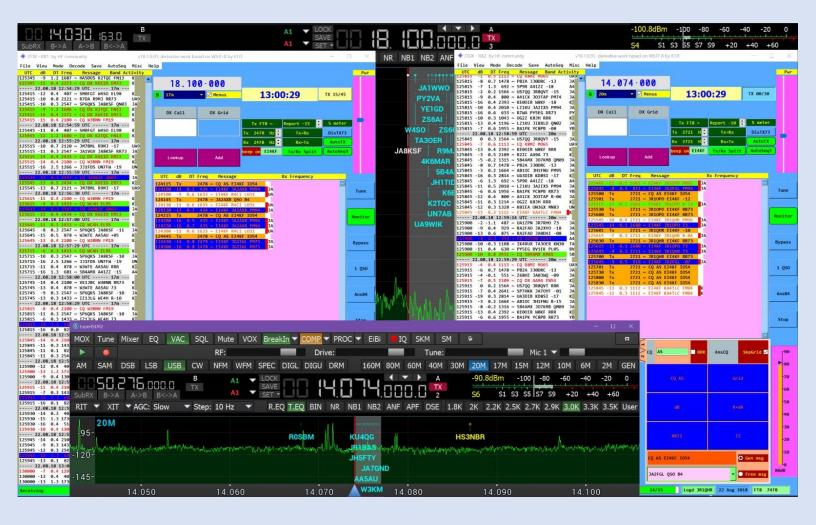
JTDX RX1 is on 17mtrs and JTDX RX2 is on 20mtrs. Stations were worked on 18.100 and then later on 14074. Normally I have the RX2 window on a separate monitor.
