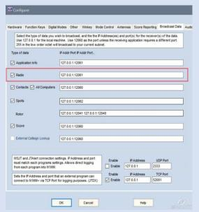
with VSElink shown in the N1MM section (6.15). A setting in the SDC TCI tab, Focus Helper, will enable window focus to be returned to N1MM+ whenever there is a click on the ESDR\* panorama, split buttons, filter, etc. or the frequency is changed. The focus will automatically return to the N1MM+ window. An additional setting has to be made in N1MM+ for focus to work. See picture left.
