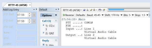
As with all digital mode software, the audio lines are Line 1 for input (receive) and Line 2 for output (transmit). PTT is on COM 10, the application side of our COM 9<>COM 10 pair we created in VAC.
