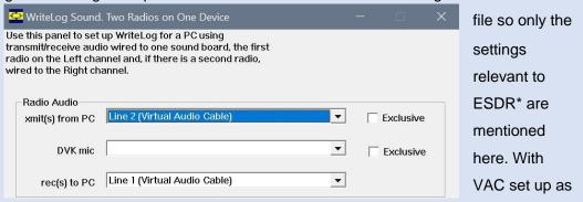
before, nominate VAC 2 for xmit(s) from PC and VAC 1 for rec(s) to PC (receive). Do not check the boxes marked Exclusive.
