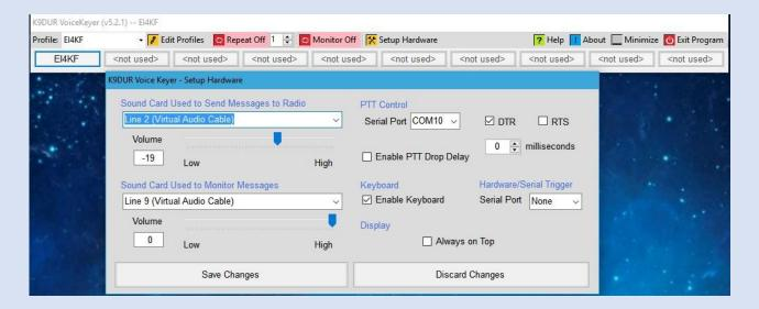
Click Setup Hardware from the main screen to open the configuration window. Set the parameters as above. The volume under Line 2 VAC controls the audio gain of the transmitted macro and should be adjusted to avoid over driving the radio. Line 9 VAC for monitoring messages and Line 8 VAC for recording messages can be set up in ESDR\* Sound Card tab
