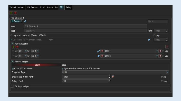
with two or more transceivers, create the appropriate number of clients. Specify the name of the connection, address and port (normally 40001). Enable the Callback TCI-Connect mode on port 40002, the same port we set up in ESDR\*. Test with the connect button. Normally the TCI link will establish automatically.
