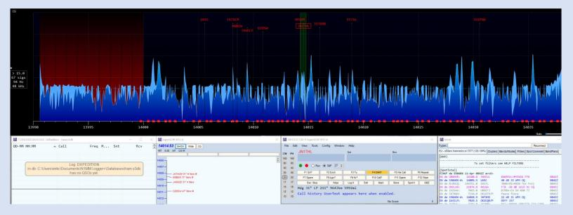
DX Spots will appear when N1MM is connected to a DXCluster in its Telnet window. Tuning the radio to a Spot on the Scope will prepare the Input window with that callsign – JN1THL in the above picture. An alternative method of interfacing ESDR\* with the N1MM Spectrum Scope can be done with SDC. See section 5.11 for details. The SDC implementation is not as good, in my opinion, but try it for comparison.
