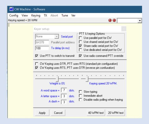
In this set up, the CW keying port is shared with CAT as with N1MM. Ensure Breakin is on in ESDR\*. The delay may need to be adjusted to the shortest possible value without truncating the signal.
