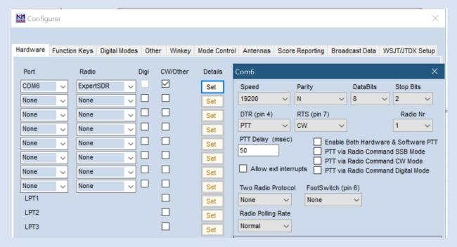
For the 2<sup>nd</sup> RX, define the COM port and Splitter COM7<>COM8 as was done for JTDX and set it up in N1MM+ in the next line down, under COM 6 in the above example. The port settings will be the same except that the 'Radio Nr' is 2. Press OK to save.
