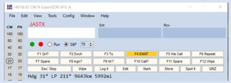
If in S&P mode, with ESM enabled, pressing 'Enter' will fill the log box and your callsign will be transmitted.
