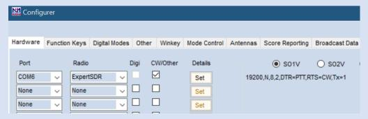
Single operator, one radio, configuration is achieved by selecting COM 6. N1MM+ includes ExpertSDR in its Radio list. Check CW/Other and then click Set and apply the parameters below.
