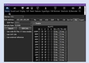
NOTE: The PA PTT delay is active for all modes except CW. In ESDR2 there is a cryptic message: "PTT switching delay disabled" but, contrary to the implication, the PTT delay in CW cannot be enabled because it does not exist. Therefore, for a hard-wired key, achieve the required delay with the Break-In setting. For COM port keying and Winkeyer, set the required delay in the software.
