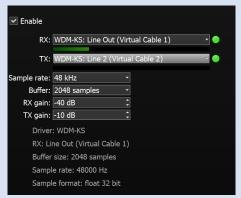
Firstly, ensure that in ESDR\* VAC settings you have configured as seen on the left. Sample Rate is 48000Hz and Sample format is 32 bit. Buffer can be reduced to 512 samples for less latency.
