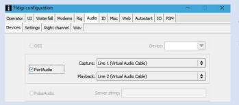
The audio set up is straightforward using the normal VAC 1 and VAC 2.
