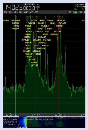
a DX Station. This shows you where the DX Station is listening. A marker can be defined instead of 599 and enabling both new and old, with different markers, will show graphically how the DX Station is working the pile – moving up or down or random. You will easily anticipate where to call to get your QSO quickly.
