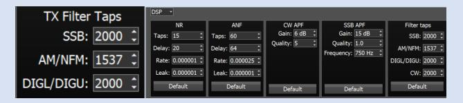
Filter Taps represent the shape of the filter. The higher number means a more rectangular
