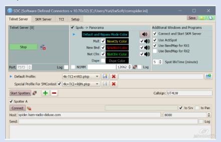
Check the LogHX connection to the SDC Telnet Server. In the Telnet Server section, the logo of the LogHX program should appear. When LogHX is connected to the SDC Telnet Server, the profile specified in 'Profile' will be selected.
