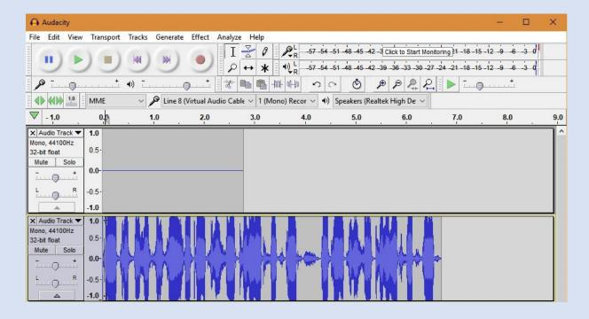
Ensure that in VAC you configured lines 8 and 9 (see the VAC section in this Manual). Configure Audacity to use Line 8 with MME as the driver. Record your mono .wav file by using your normal radio microphone with the radio in TX but power out at zero. Using Audacity, edit the file to remove non-audio time before and after the message. Save the .wav file and transfer to the K9DUR folder. Macros are set in K9DUR profiles.
