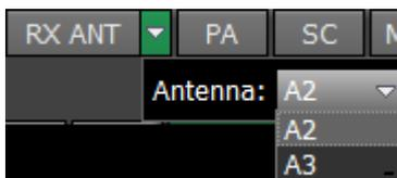
**RX ANT** button enables receiving on the selected antenna input, which is selected in the drop-down menu. You cannot select the antenna input as **RX ONLY** if it's selected for TX.
