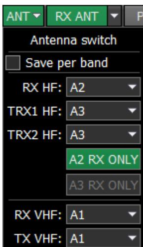
**Antenna switch** menu. This menu allows you to lock the required HF/VHF antenna input **only for RX**. When the certain HF/VHF antenna input is locked for RX you cannot select it for TX.
