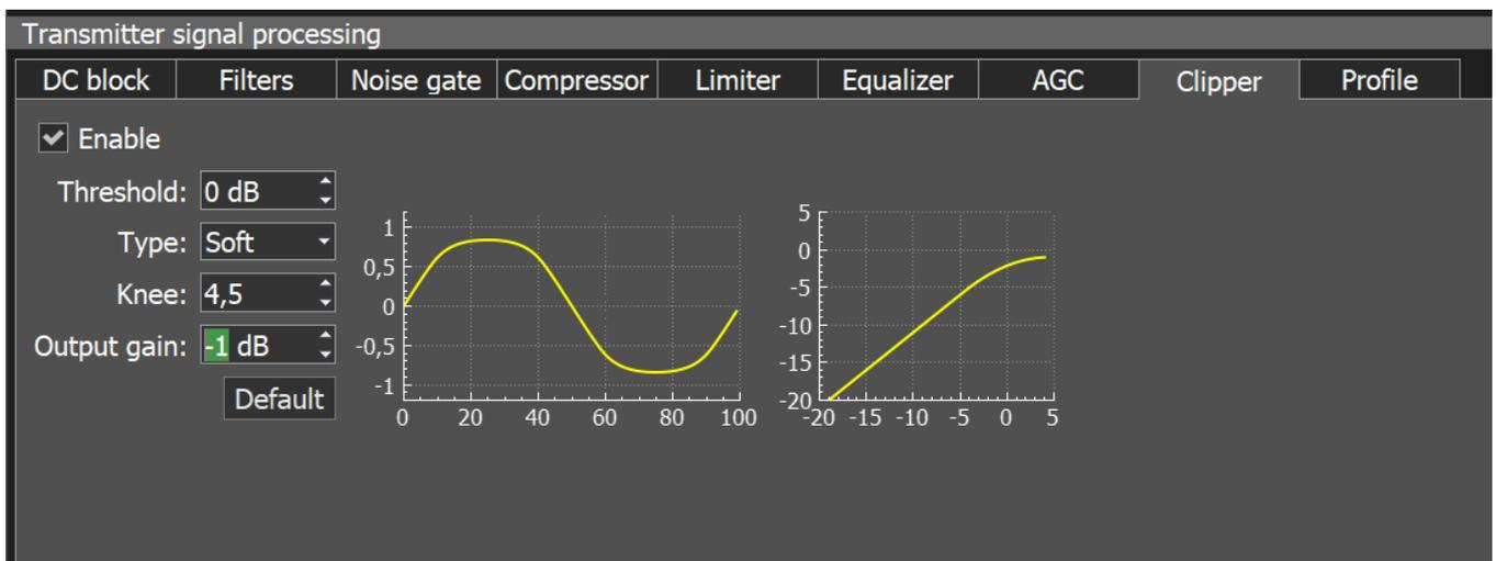
**Clipping** is a form of waveform distortion that occurs when the output Voltage exceeds **Threshold**. Visually (on oscilloscope) it looks like altered signal peaks, you can hear it as splutters and cracks. **Clipper** reduces signals peak-factor and increases overall power, but distorts the signal.
