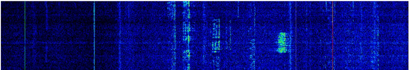
Waterfall graphic - timed spectrum scope in the format: amplitude - brightness, frequency - horizontal, time - vertical. The comfortable settings are set by default, but you can change them if necessary (more details in [Waterfall tab](#)<sup>75</sup>).
