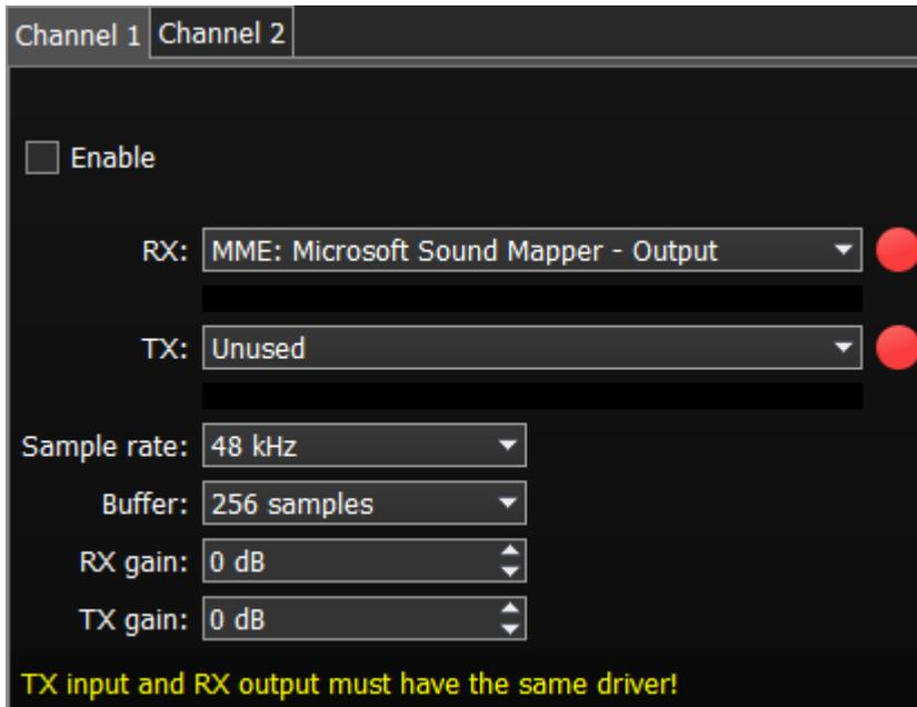
For each program receiver (RX1, RX2) you can set the virtual audio cable on the corresponding tab **Channel 1** and **Channel 2**.
