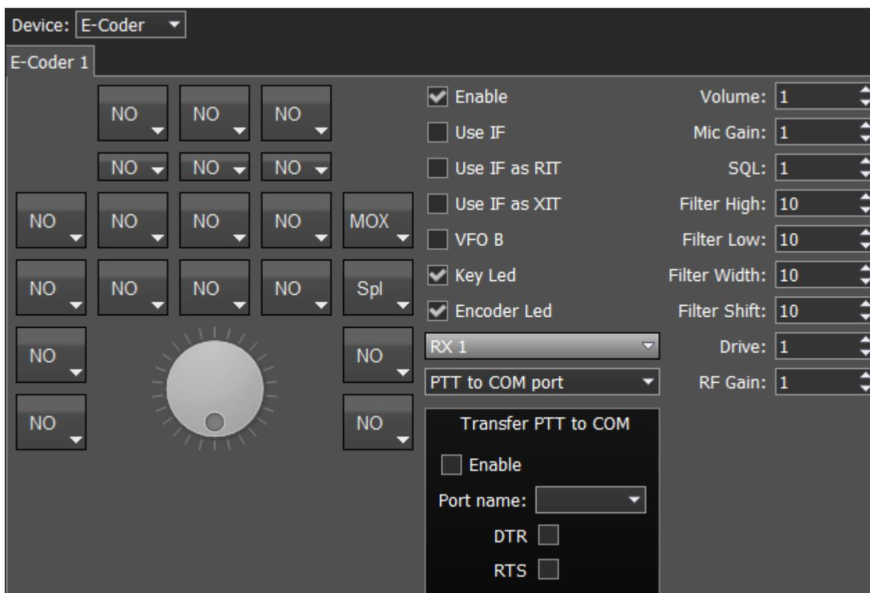
In the left part of the menu you can see the schematic picture of the E-Coder panel with buttons and knobs. Press any button, you'll see the list of the available functions.
