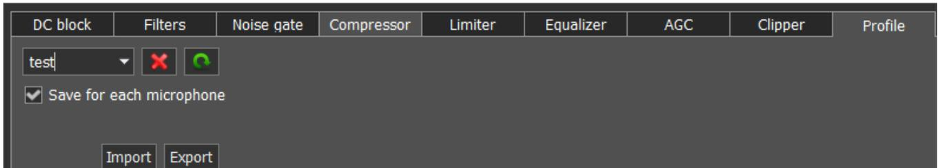
In the **Profile** tab, you can save settings of the whole TX processing module in a separate module, independent from the main software profile. Load PROC settings from a file by pressing the **Import** button and save a profile in a file by pressing the **Export** button.
