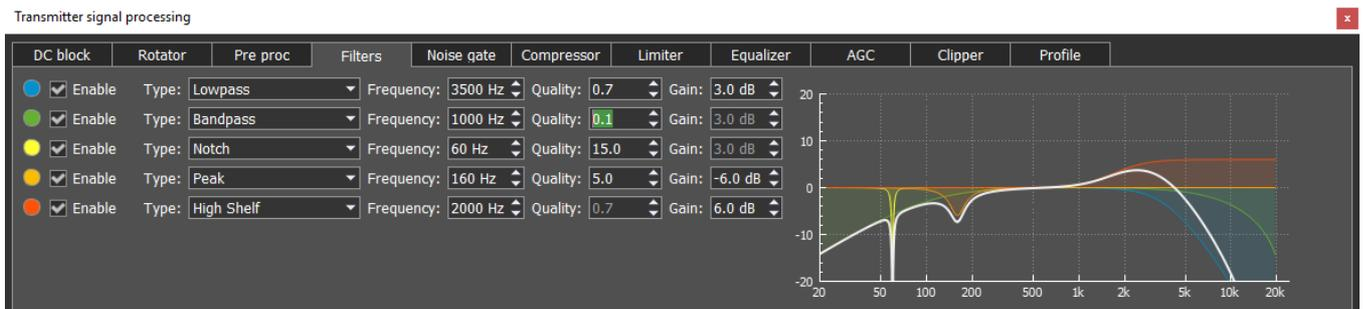
**Parametric filter module** with graphic display of the summed AFC (amplitude-frequency characteristic - white line) and AFC of each filter. Simultaneously you can use up to 5 filters. Available filter types:
