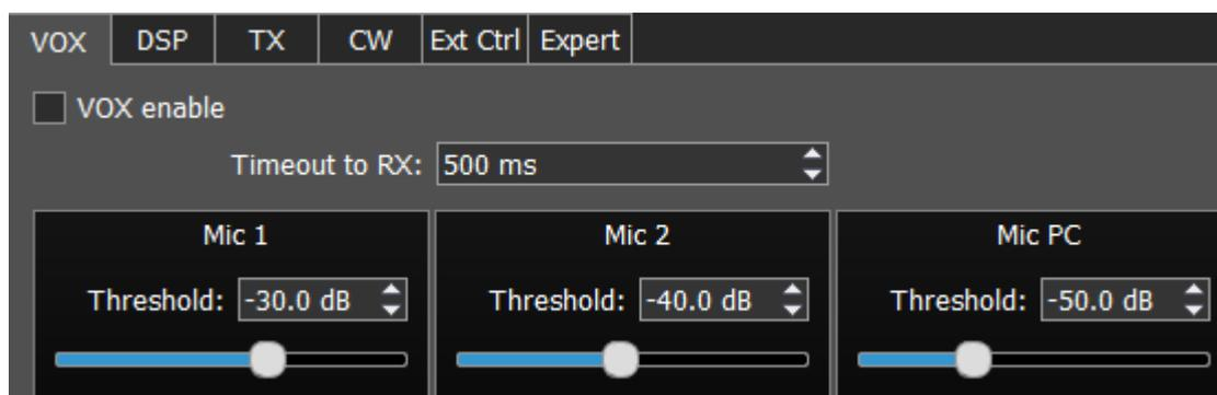
VOX system triggers when the microphones voice signal exceeds the **Threshold**. The **Threshold** could be set for each microphone individually.
