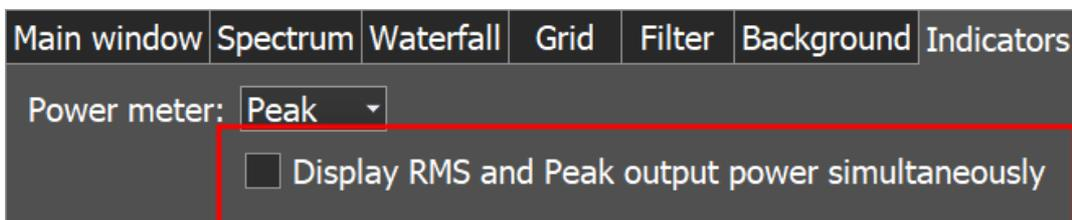
In the Peak/RMS drop-down menu you set the type of output power which is displayed on the Power and S-meters. What you check there always displayed as text on the Power meter.
