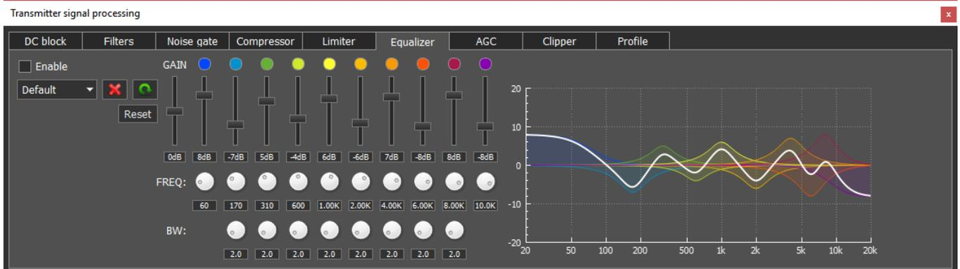
Parametric equalizer module with graphic display of the summed AFC (white line) and AFC of each equalizer. Each equalizer has independent set of controls: the center or primary frequency (**FREQ**), bandwidth (**BW**) and AFC level (boost or cut) - vertical slider. Press right mouse button on any control element to set it to the default value. Thus, using the parametric equalizer you can perform the finest tuning on any required frequency.
