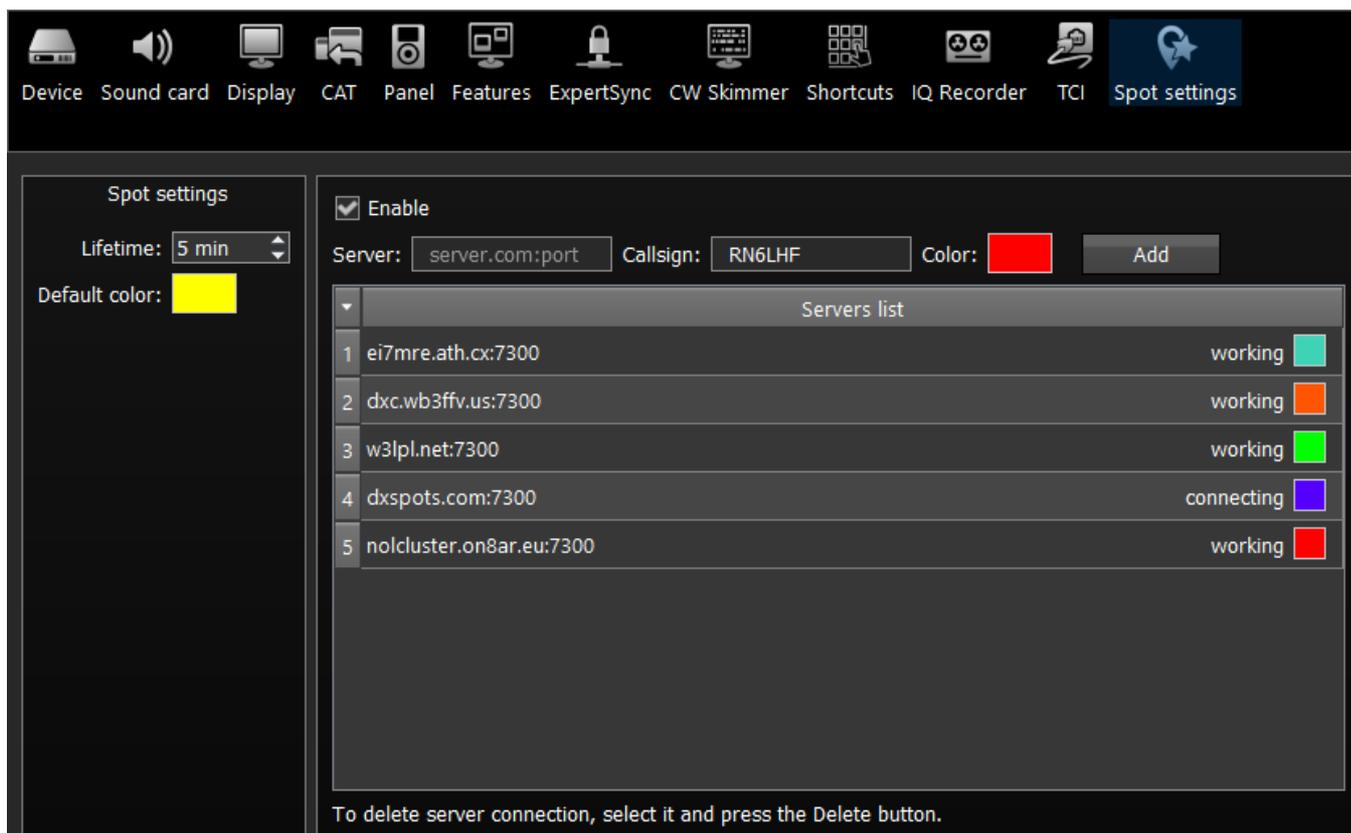
In the **Spot settings** section (left part of the menu) you can set up **Lifetime** and **Default color** for spots received from CW Skimmer.
