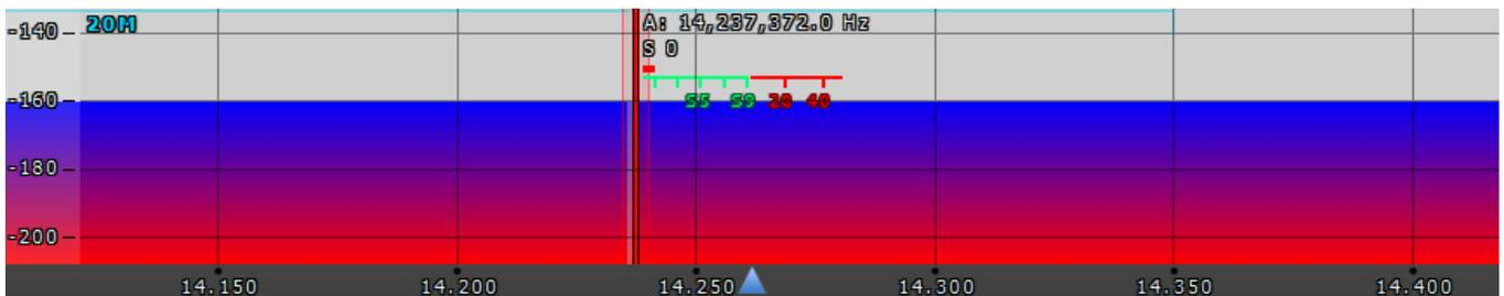
In this window, you can see the spectrum, with the sample rate from 39 up to 312 kHz (adjustable by User) and the RX filter to tune and listen to the stations.
