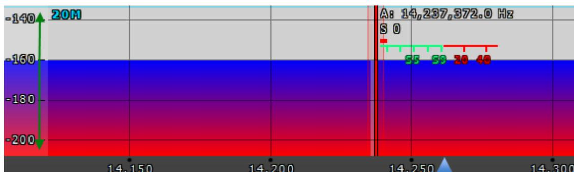
The horizontal scale between the spectrum scope and waterfall shows the frequency of the certain point on the spectrum. If you move the mouse cursor over the horizontal scale a hand will appear. Press and hold the right mouse button, then move it left/right to zoom in/out the panorama or press and hold the left mouse button, then move it up/down to change the ratio of the spectrum to waterfall.
