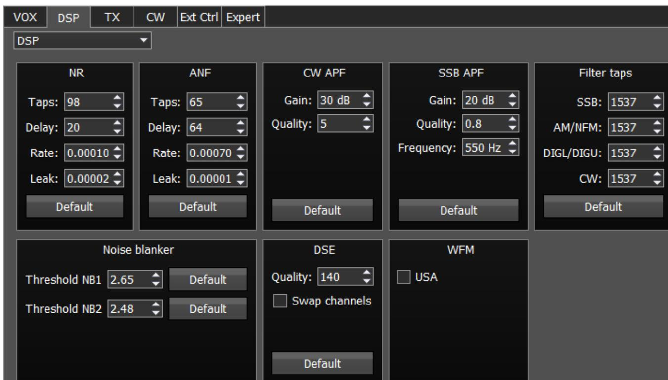
**NR** - Noise Reduction, removes the white noise. This is a special adaptive filter, which removes any abnormal noises from the air in the RX filter band.
