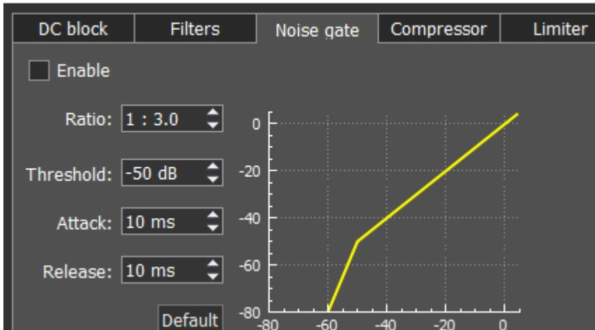
**Noise gate** or **gate**, removes signals below **Threshold** level. Usually it is used to reduce the noise in pauses.
