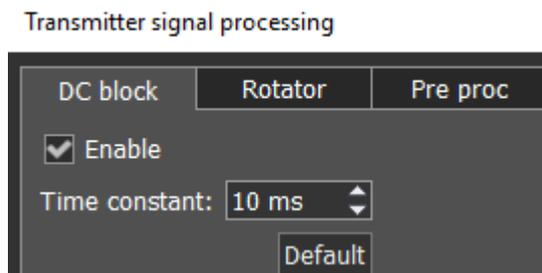
**DC block's** purpose is to effectively remove **Time constant** in the microphone signal. Changing of **Time constant** influence quality of the applied filter. You can test it by increasing or decreasing **Time constant** value in 1-10 ms range, you'll notice low frequencies reduction with 1 ms value and amplifying with 10 ms value.
