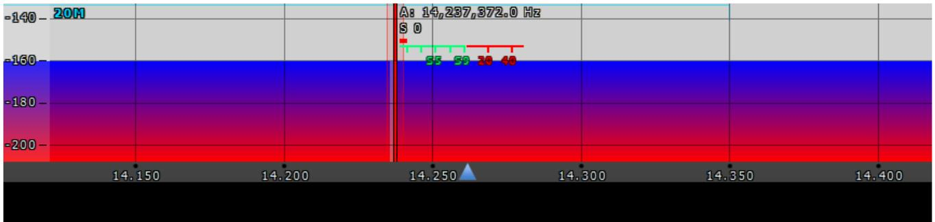
The panorama consists of two parts separated by the horizontal scale: 1) Spectrum Scope and 2) Waterfall.
