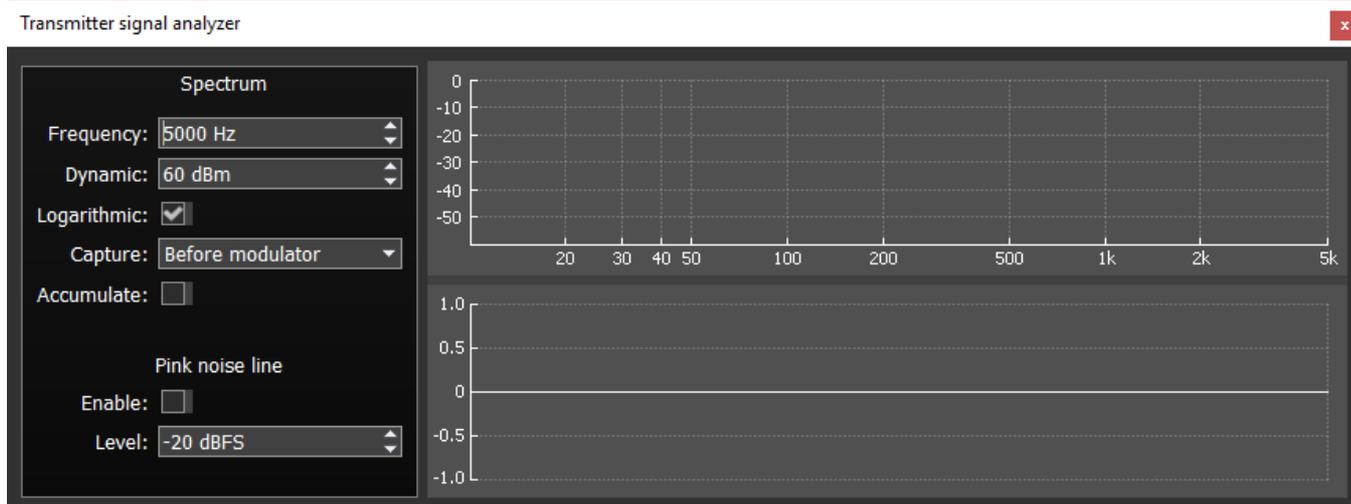
**Frequency** - top limit of the horizontal (frequency) scale of the transmitter.
