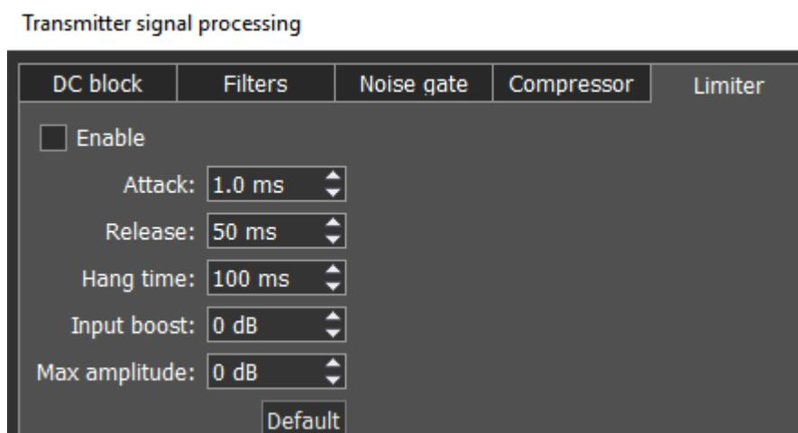
**Limiter** - is used to limit dynamic range, when signal exceeds **Maximum Amplitude** value. In most cases used to avoid overload (clipping) and suppression of short-term level peaks, while signal dynamic range is being leveled. As a rule, limiter is used along with increasing the input level on the **Input Boost** value, this technique increases overall signal level, while preventing distortion.
