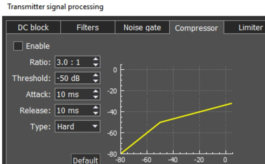
**Compressor** - is used to reduce
