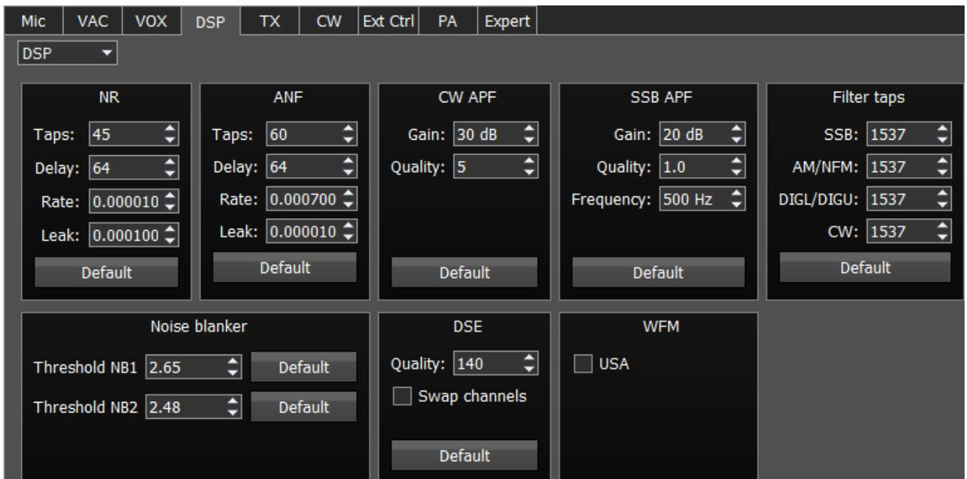
**NR** - Noise Reduction, removes the white noise. This is a special adaptive filter, which removes any abnormal noises from the air in the RX filter band.
