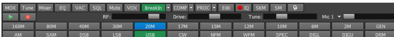
**MOX** - enable/disable manually operated transmit mode (**MOX**).
