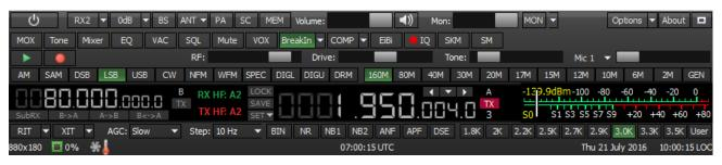
¾ of the software window is occupied by the panorama: spectrum scope and waterfall. The waterfall is a convenient feature which allows you to observe the signals' changing dynamic in time.
