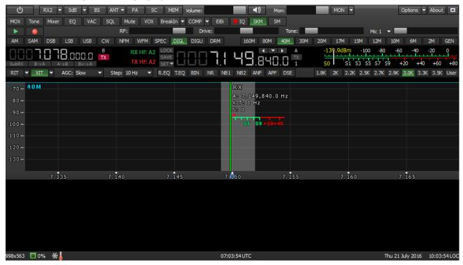
1/4 of the software window is occupied by the functional buttons and operational indicators (frequency, S-meter etc.)
