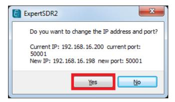
If everything was done correctly and IP address is set, the new value of IP will be displayed in the SDR Address box
