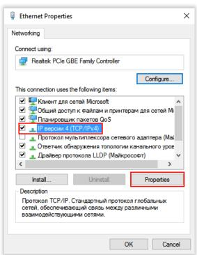
Set the IP-address to 192.168.16.50 and subnet mask to 255.255.255.0 as it is shown below. These are the PC's network card parameters. Instead of the figure 50 in the IPaddress you may set any number, except 255 or 200. Transceiver IP-address is
