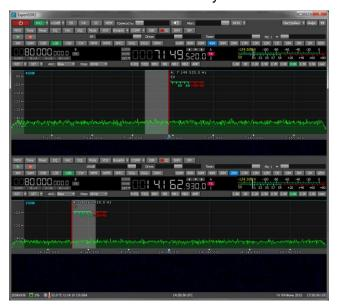
3) Two receivers separately. This way each receiver has its own window and can be moved easily along the screen.
