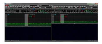
2) Vertical arrangement of one receiver above the other. Such arrangement is convenient when you use an old big monitor with 4:3 aspect ratio or modern monitor turned vertically.
