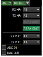
**RX antenna** menu. This menu allows you to lock the required HF antenna input **only for RX**. When the certain HF antenna input is locked for RX you **cannot** select it for TX.
