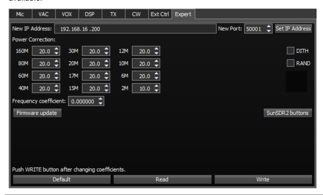
Note! All settings in this tab are stored in the transceiver's energy independent memory. After setting the required values, set/unset checkboxes, press the Write button to store the info in the memory.
