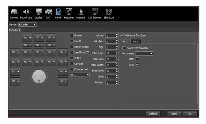
In the left part of the menu you can see the schematic picture of the E-Coder panel with buttons and knobs. Press any button, you'll see the list of the available functions.
