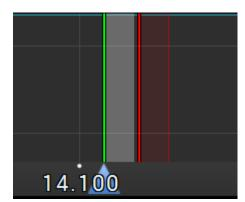
XIT offset in the TX mode means that receiving will be held on the tuned frequency and transmission frequency will differ by the offset value. Offset is displayed as a translucent band on the spectrum scope. Tuned RX frequency displayed as the green line. TX frequency displayed as the red line with the filter band (on the picture you can see the USB mode).
