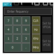
SET - manual input of the frequency to VFO A or VFO B.
