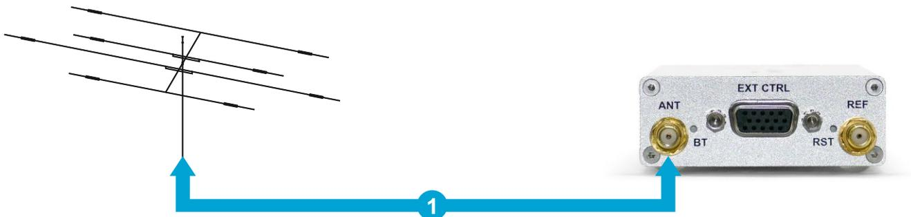
1. Connect antenna to the receiver's antenna input.
