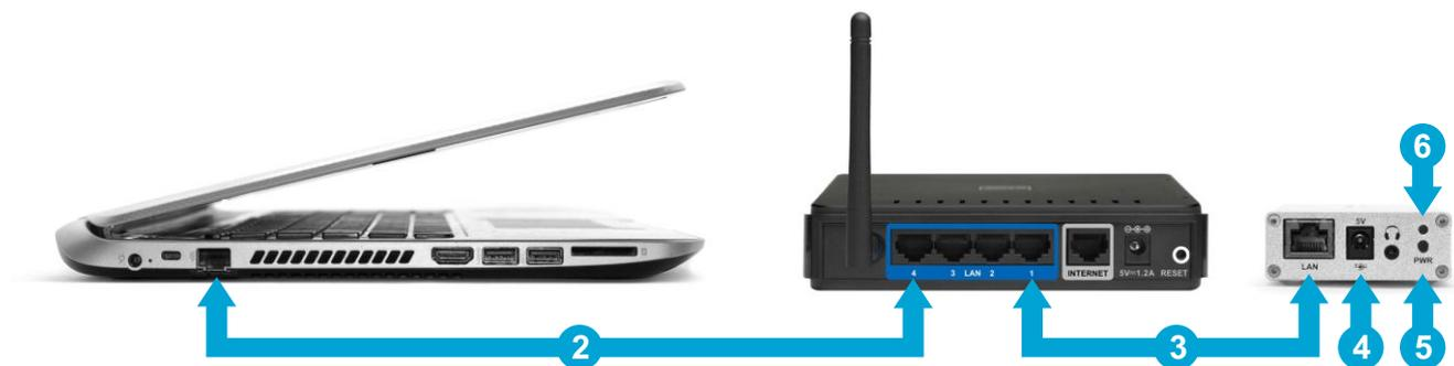
2. Connect PC to the router using LAN cable
